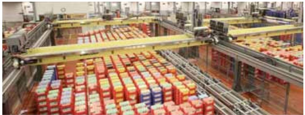
► conveyed by monorail but to a special storage area where they are positioned on dolly conveyors in buffer lanes. Products received from elsewhere are registered on the warehouse management system (WMS) and then transferred by fork-lift truck, with palletized products and those in cardboard cases going to the semi-automatic picking system but stacks of crates and roll-in containers being delivered to the monorail for transport to the MultiPick and roll-in storage areas respectively.
